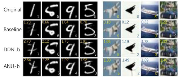
Figure 6: Adversarial examples against three models: baseline, DDN-based, ANU-based defenses. Text on top of each image indicates L_2 norm of the noise \|\delta\|_2 . Text on bottom indicates the predicted class 2 .
