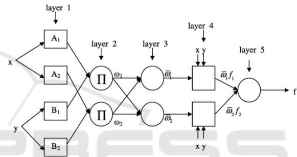
Figure 2: ANFIS structure (Guner et al., 2011).
