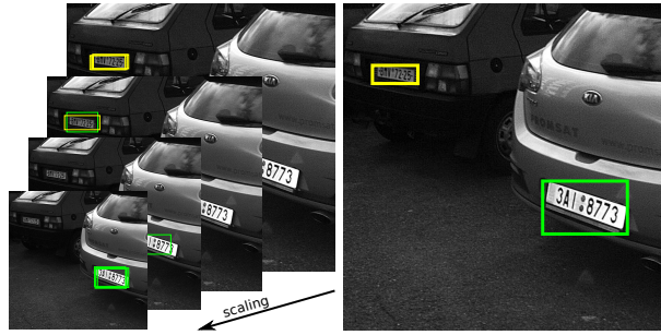
Figure 2: (left) Image scales and objects detected by the classifiers. (right) Final detections after non-maximum suppression. The classifiers are color-coded, the yellow one detects license plates almost aligned, the green one detects slightly tilted license plates.
