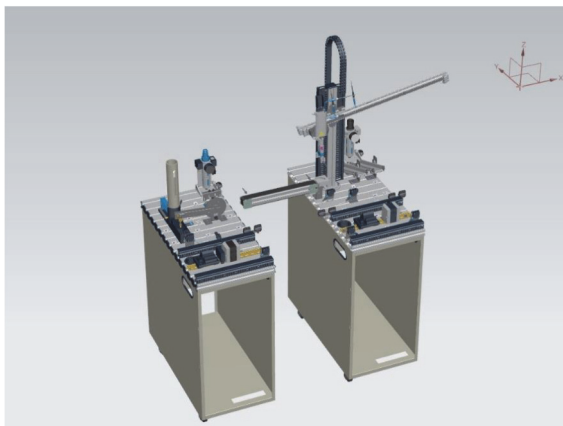
Figure 13: Digital twin cap supply station.
