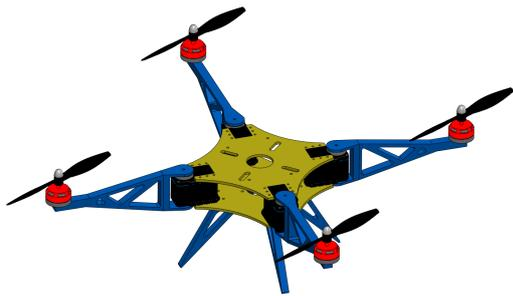
Figure 1: Design of our proposed quadrotor, able to change its configuration while flying. Each rotor is connected to a rotating arm. Each rotating arm is connected to a servomotor and it can rotate independently.
