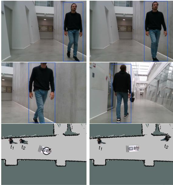
Figure 1: Two problems arising when using 2D tracking on a mobile robot. Left column shows camera images before and after the robot has rotated, causing a shift in the center pixel of the person. Right column shows a person transitioning from one camera to another, which is undefined in image coordinates. Both are non-issues when tracking the 3D coordinates in the map frame. Here the before and after are shown as time step  $t_1$  and  $t_2$ .
