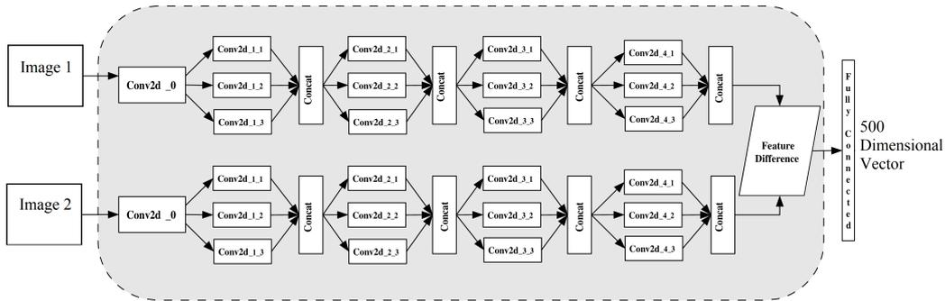
Figure 2: Insight view of the proposed Siamese Multi-scale Network (SMSNet) architecture. First layer of convolution is unaffected of dilation parameters. All other layers are dilated with rate 1,2,3 and feature aggregation has been done after each convolution layer in form of concatenation. Feature difference is computed after 4<sup>th</sup> convolution layer.
