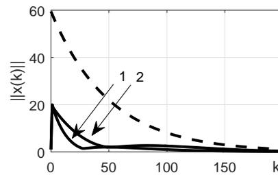
Figure 5: Norm of free motion and upper bound estimation of the discrete-time system with unpredictable delay.
