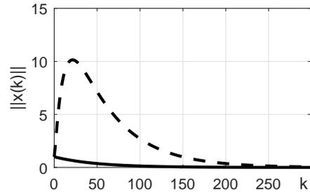
Figure 1: Norm of free motion of a stable discrete-time system for different descriptions of the state matrix  $\mathbf{F}_1$  (dashed line) and  $\mathbf{F}_2$  (solid line).
