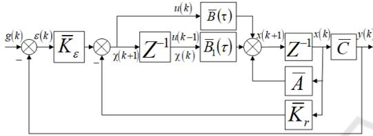
Figure 2: Block diagram of system with unpredictable delay in control.
