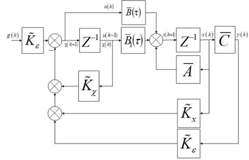
Figure 3: Block diagram of system with predictable delay in control.
