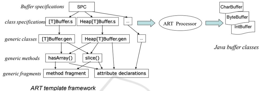
Figure 7: Non-redundant representation of Buffer classes in ART/Java.
