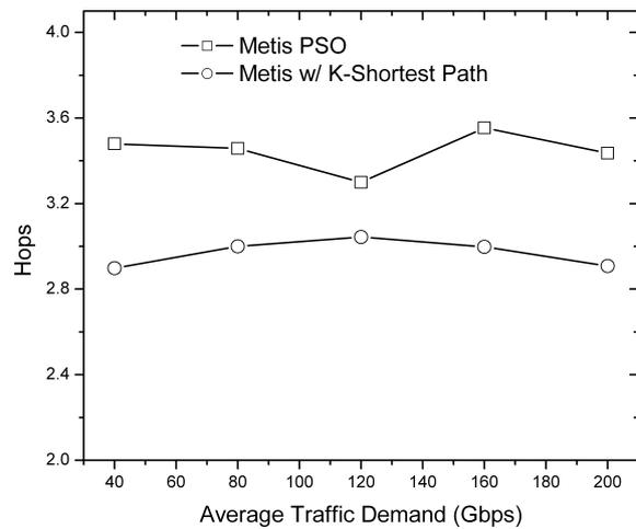
Figure 7: Hop-count according to increased traffic demand.
