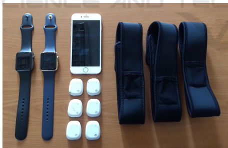
Figure 2: Data capture system. Two Apple watches on the left, an iPhone 7 and 6 MMR devices in the middle. Three velcro sleeves on the right.
