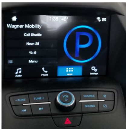
Figure 10: Integration of mobile application with vehicle using SmartDeviceLink.
