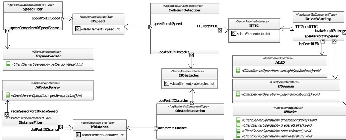
Figure 5: AEBS software components as seen in the software component diagram modeled in Rhapsody.
