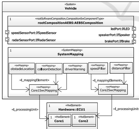
Figure 6: System diagram containing the system mapping and the root software composition.
