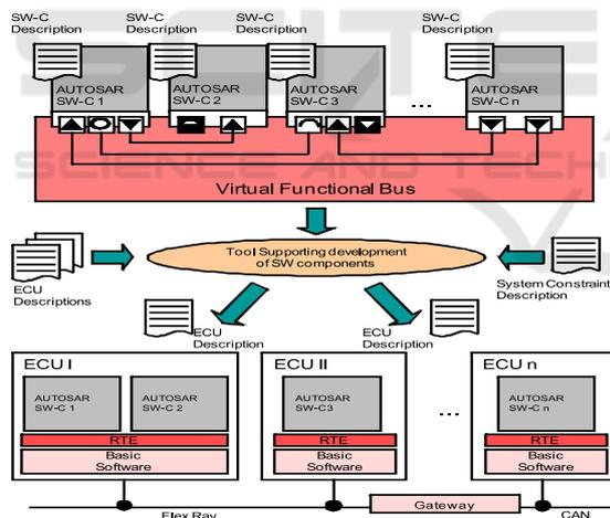
Figure 2: Various components of AUTOSAR framework & mapping of Software Components (SW-Cs) to ECUs.
