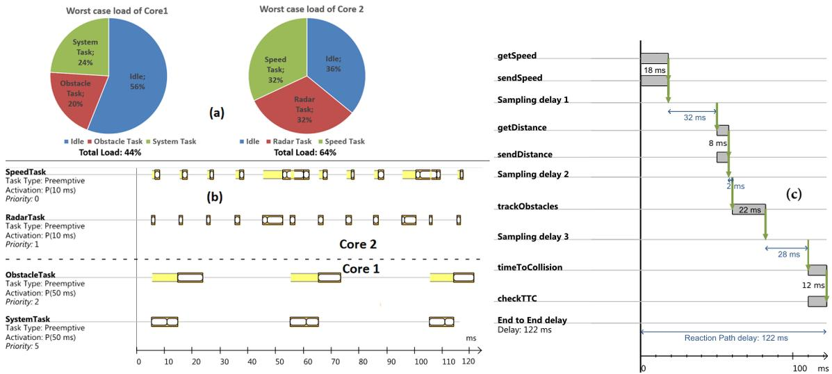
Figure 11: (a) Worst case load of processing cores 1 & 2 (b) Exemplary task scheduling for system distribution analysis and (c) Worst case response time for the causal event chain `systemEventChain` modeled in use case (ref. section 3.5.1).
