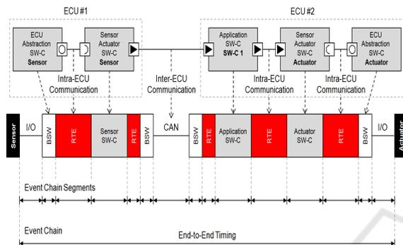
Figure 3: End-To-End timing of a AUTOSAR-based causal event chain (AUTOSAR, 2017).
