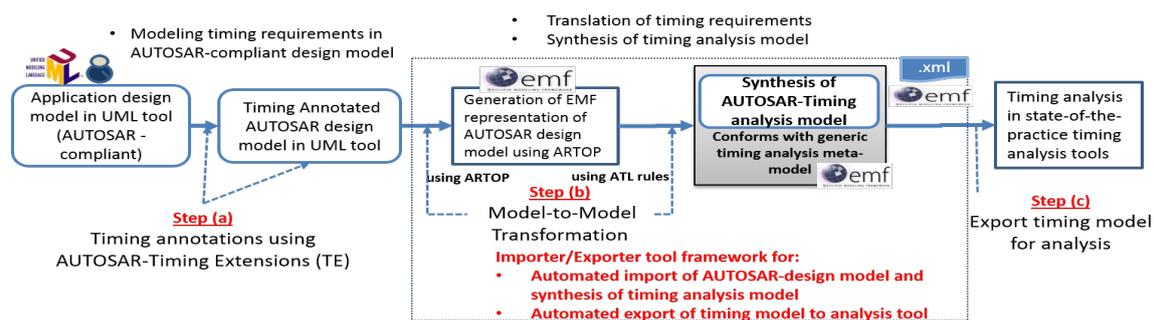
Figure 1: Systematic series of steps for early timing analysis in AUTOSAR-based ESE (introduced in (Iyengar et al., 2020)).
