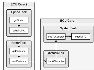
Figure 7: AEBS architecture and end-to-end execution path.
