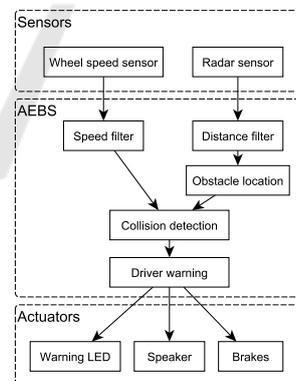
Figure 4: Control flow and modules of the AEBS.
