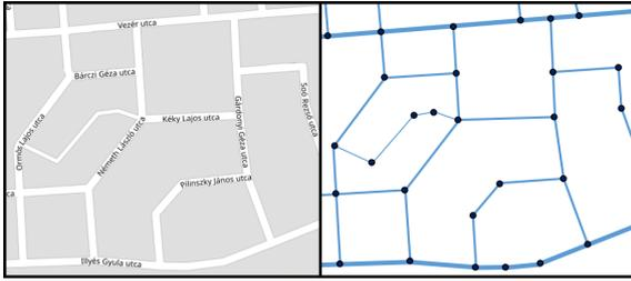
Figure 1: The urban road map of Debrecen (left) was converted to a weighted graph connecting real geographical locations with different kinds of straight road segments (right).
