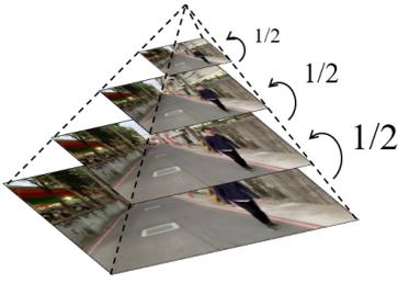
Figure 3: The pyramid of image. The full image resolution is taken at the bottom level.
