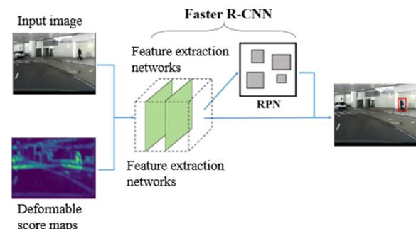
Figure 7: The framework of detecting pedestrians with deformable score maps on the Faster R-CNN architecture.
