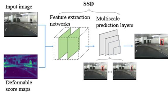
Figure 6: The framework of detecting pedestrians with deformable score maps on the SSD architecture.
