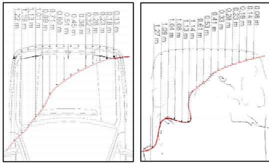
Figure 8: Skoda Felicia frontal impact – top-view (left) vs. scanner (right).
