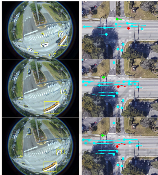
Figure 9: Qualitative Results of Object Trajectories Mapping to Satellite Map. left: Tracking in Fisheye Video. right: Trajectories after Mapping. Different Color Represents Different Object Class (Red for Bus, Green for Pedestrian, Blue for Car).
