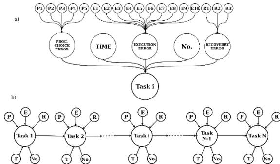
Figure 5: Graphs of the model: a) Subgraph that models probability of error occurrence in Task i; b) Graph of simulated activity with concatenated tasks.
