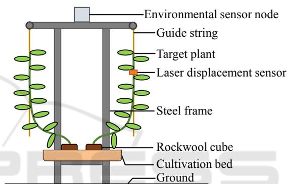
(b) Layout of measurement sensors.
