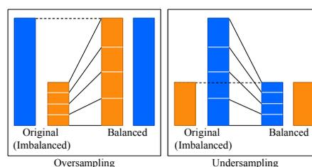
Figure 1: Addressing imbalanced data with resampling.
