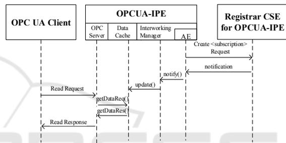
Figure 6: Read Service using Data Cache.
