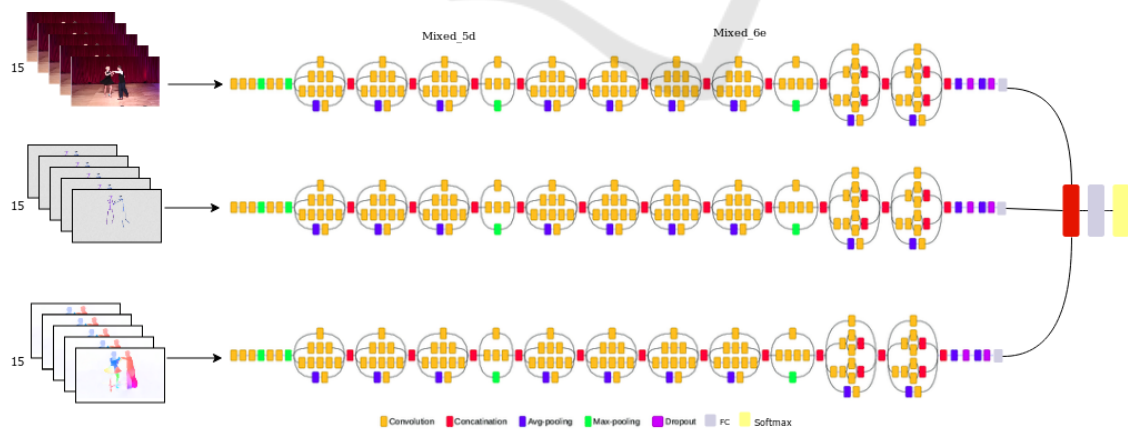
Figure 3: The high level architecture diagram of Three-stream Temporal Inception core CNN.
