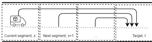
Figure 4: Multi-Step Gradual Prediction Approach. Delays from the Current Segment Are Used to Adjust Expected Travel Time to the Destination Segment.
