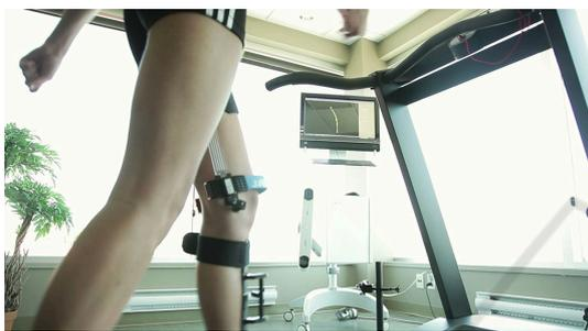
Figure 1: Knee kinematic acquisition system.
