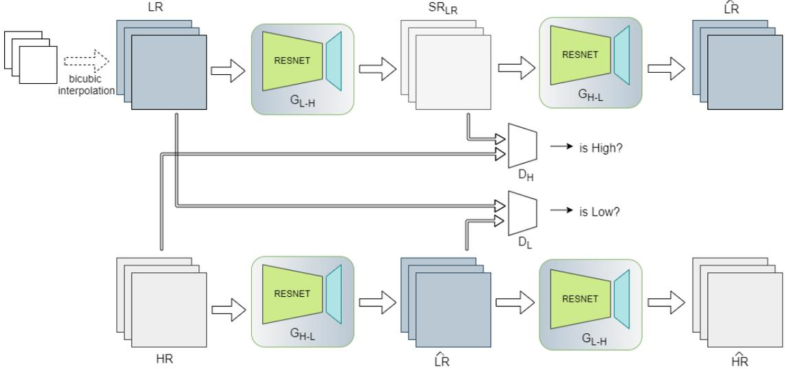
Figure 6: Proposed CycleGAN architecture using 6 residual blocks ResNet;  $G_{L-H}$  and  $G_{H-L}$  represent generators from lower to higher and from higher to lower resolution respectively.  $D_H$  and  $D_L$  represent the discriminator for each resolution.
