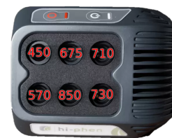
Figure 1: Disposition of each band on the Airphen multi-sensors camera.
