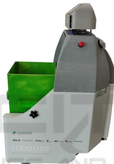
Figure 3: The SMOOTH robot docked with the bin used for use case 1 of the SMOOTH project.
