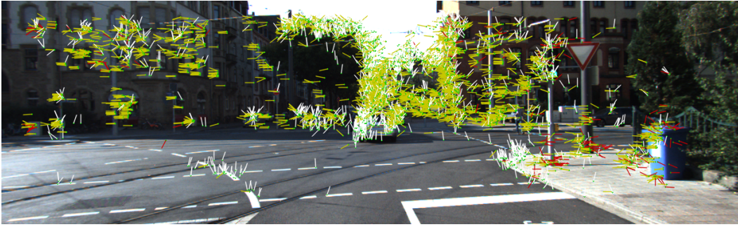
Figure 3: Estimated surface normals visualized in an image of one of the KITTI (Geiger et al., 2012) sequences. Yellow, white and red coordinates are used for horizontal, vertical and perpendicular, to the image plane, directions. Best viewed in color.
