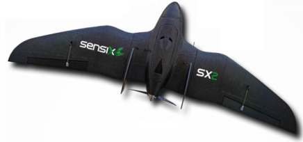
Figure 3: Micro UAV SX2 by Sensix Innovations.
