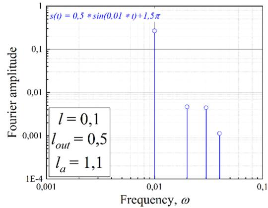
Figure 6: Fourier spectrum of the output signal from real ReLU transfer function during of transmitting a harmonic signal for the case of an operating point at the linear part of the transfer characteristic.
