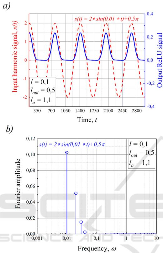
Figure 4: An example of transmitting a harmonic signal through the real ReLU when selecting an operating point at the zero part of the transfer characteristic (a) and the Fourier spectrum of the output signal (b).
