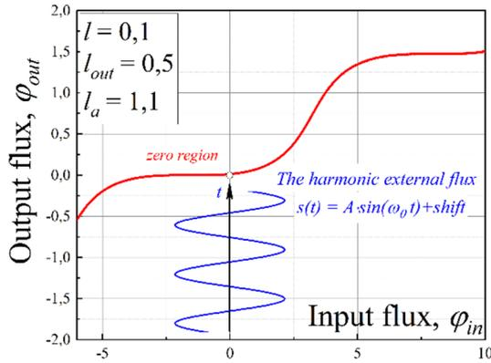
Figure 2: Illustration of applying a simple harmonic signal to the input of ReLU scheme after selection of an operating point at the end of the zero section.
