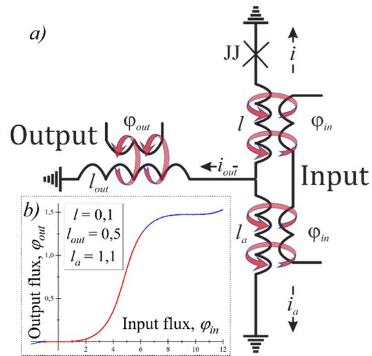
Figure 1: a) Principal scheme of superconducting neuron. b) Transfer function of neuron (blue line) and softmax function or leaky ReLU (red line) for  $l=0.1$ ,  $l_{out}=0.5$  and  $l_a=1.1$ .
