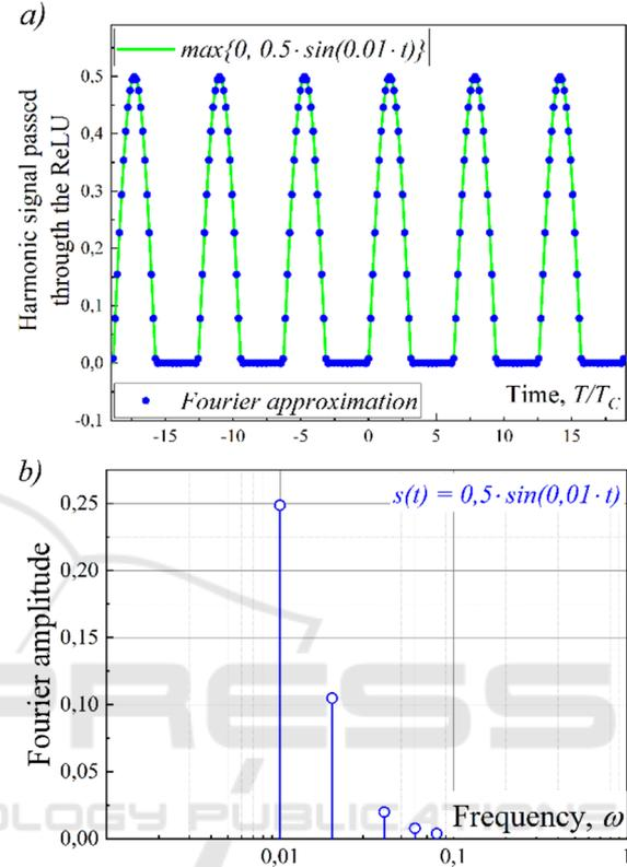
Figure 3: The result of passing through a mathematical ReLU a simple harmonic signal and its approximation using the Fourier series (a) and the Fourier spectrum of the output signal (b).
