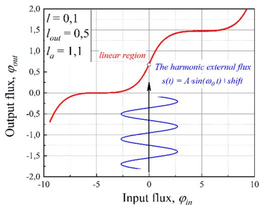
Figure 5: Illustration of applying a simple harmonic signal to the input of ReLU scheme when selecting an operating point in the middle of the linear section.
