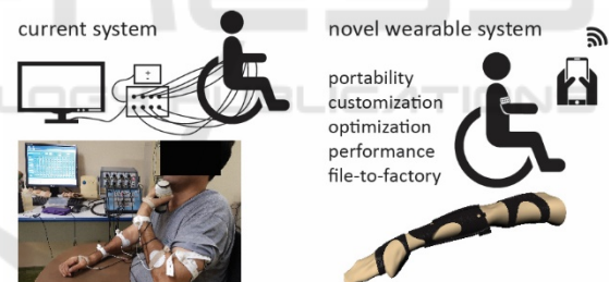
Figure 1: The picture of the left shows the current NMES system applied to the patient of the outpatient department from the Clinic Hospital (HC), of the State University of Campinas (Unicamp), Brazil versus the picture of the right that shows the proposed novel wearable system.
