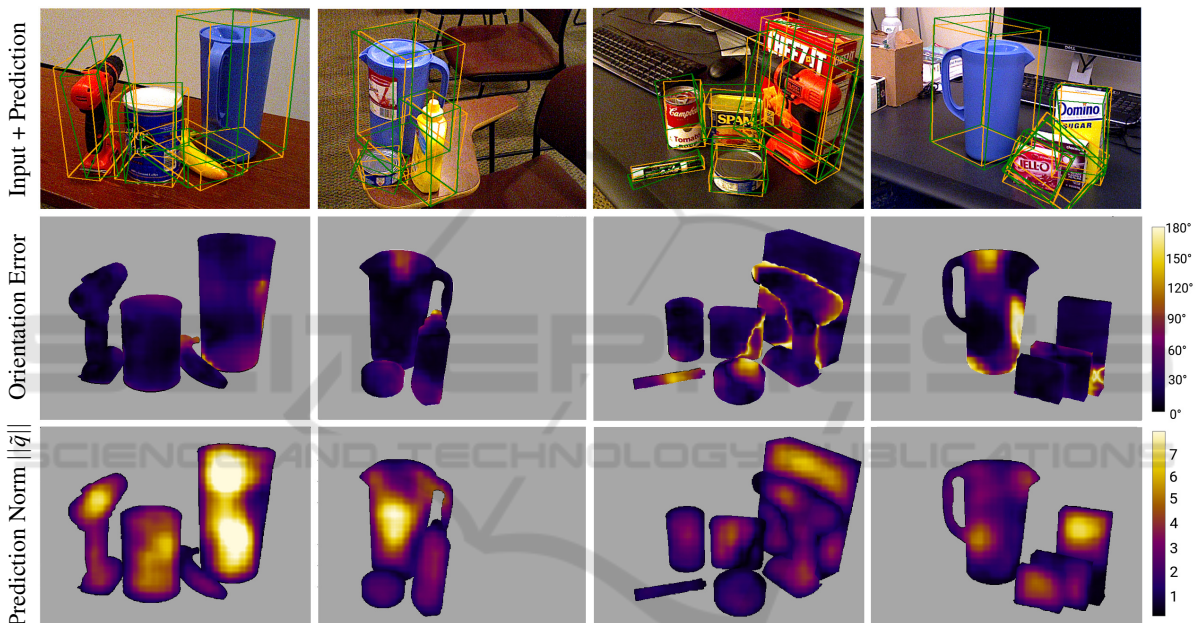
Figure 3: Qualitative results from ConvPoseCNN L2 on the YCB-Video test set. Top: The orange boxes show the ground truth bounding boxes, the green boxes the 6D pose prediction. Middle: Angular error of the dense quaternion prediction \tilde{q} w.r.t. ground truth, masked by ground truth segmentation. Bottom: Quaternion prediction norm \|\tilde{q}\| before normalization. This measure is used for weighted aggregation. Note that the prediction norm is low in high-error regions and high in regions that are far from occlusions and feature-rich.
