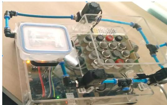
Figure 2: E-NOSE prototype developed by UIS in (Ruiz Jiménez, 2018).
