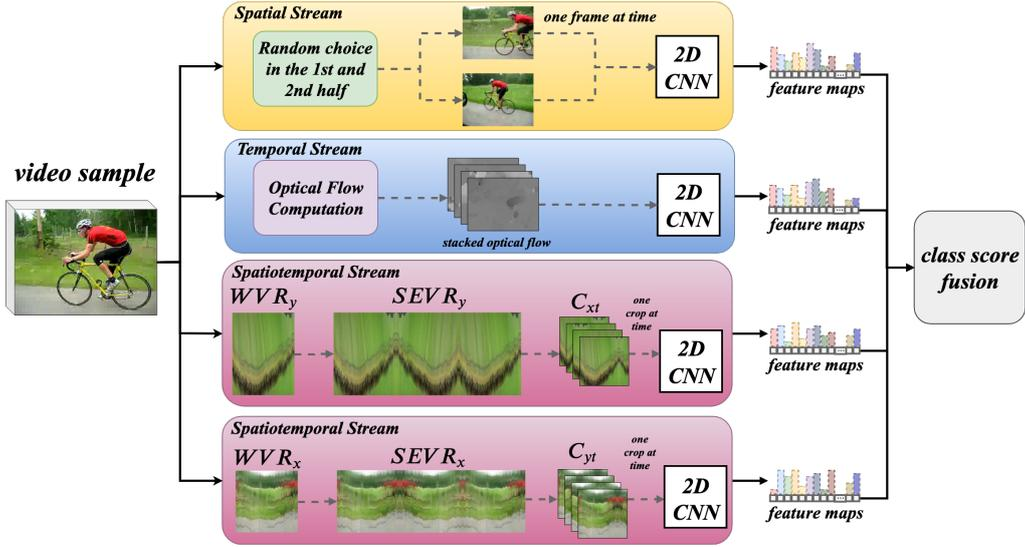
Figure 1: Final multi-stream architecture. The training of each stream is performed individually, and a weighted sum of the feature maps determines a descriptor utilized in the final classification.
