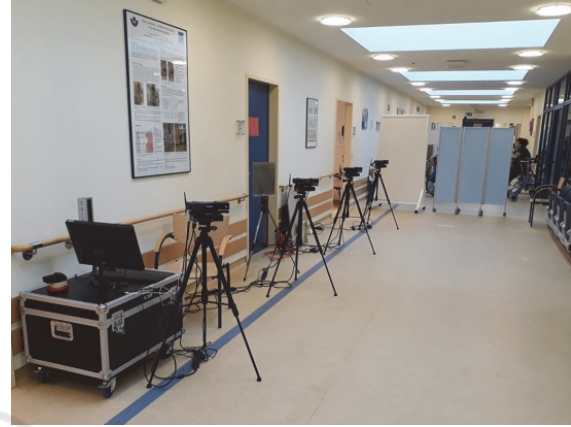
Figure 10: Walking corridor with four sensors on tripods.
