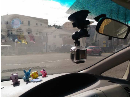
Figure 7: Experimental setup of in-vehicle camera and reflection on windshield.
