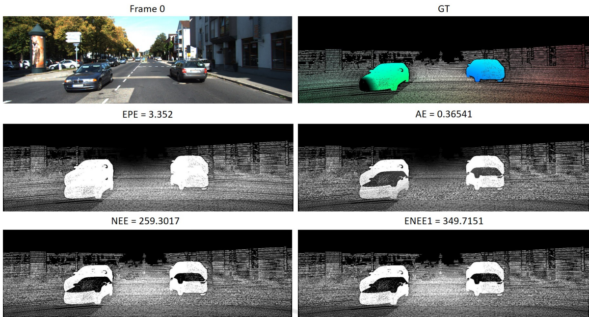
Figure 10: Sample image from KITTI's dataset, the corresponding ground truth and the visualization of motion error for four different error metrics (EPE, AE, NEE and ENEE1) between ground truth and modified ground truth when GT pixels are shifted vertically by -50 pixels.
