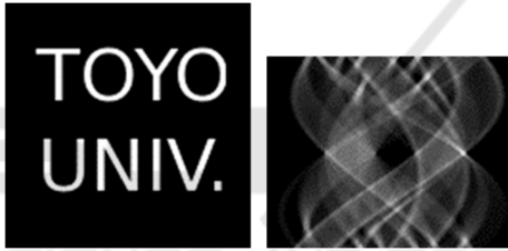
Figure 3: The original test image 1 (128×128pixel, 8bpp) and its projection data (Sinogram: 128 Detectors, 100 Views and 8bpp).
