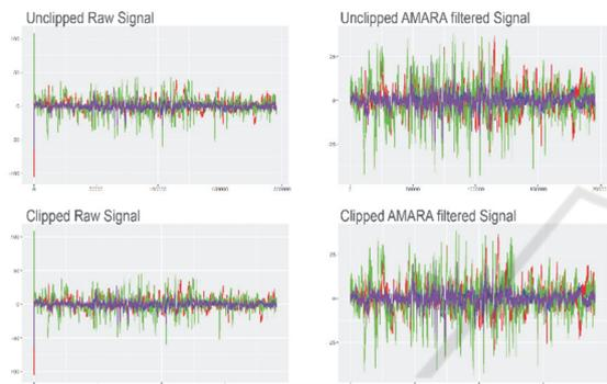
Figure 9: Raw (left) and AMARA-filtered (right) signal for a single subject before (top) and after (bottom) the clipping procedure.
