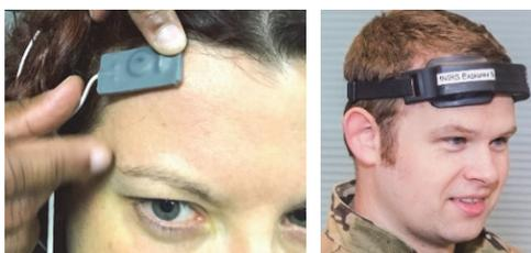
Figure 2: fNIRS Pioneer sensor to demonstrate clear position on the forehead (left) and fNIRS Explorer as it was positioned for this study (right).
