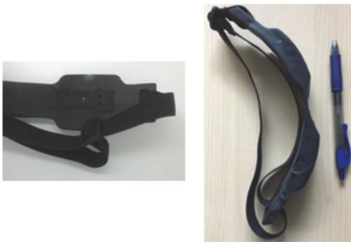
Figure 1: fNIRS Explorer sensor, bottom view of sensor that gets placed against the person's forehead (left), and side view of the sensor with a pen shown for scale (right).
