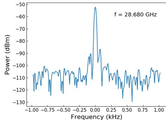
Figure 6: Repetition-rate of the frequency comb with a pump modulated at 28.68 GHz.
