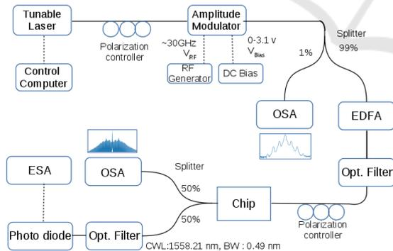
Figure 1: Experiment setup for frequency comb generation.
