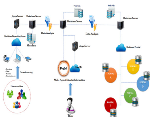
Figure 4. Integrated Design of Application for Disaster Information System
