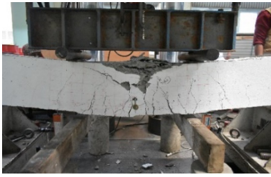
Figure 7: Element precast hybrid beam BU226 has tested
