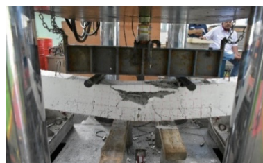
Figure 6: Element precast hybrid beam BU228 has tested
