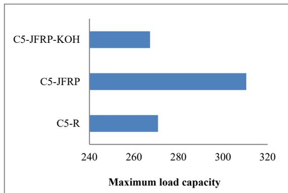
Figure 2: Maximum load capacity for specimens reinforced with fibers treated in 2% of KOH solution
