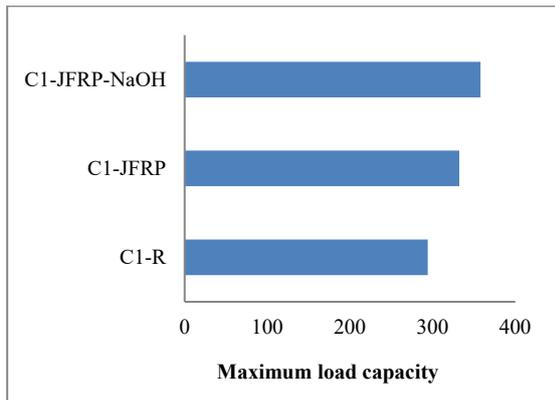
Figure 1: Maximum load capacity for specimens reinforced with fibers treated in 4% of NaOH solution.
