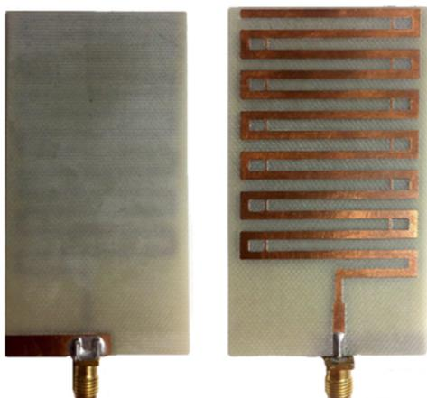
Figure 17: The fabricated antenna (Front view and Back view).
