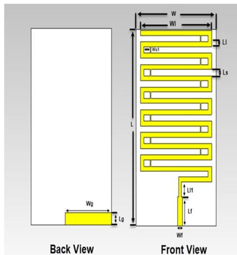
Figure 11: Proposed meander line monopole antenna.
