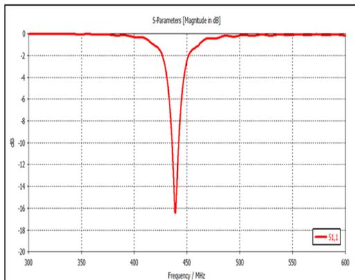
Figure 12: The return loss and operating frequency of the proposed antenna.
