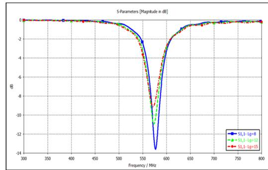
Figure 6: The effect of the ground plane length on the return loss.
