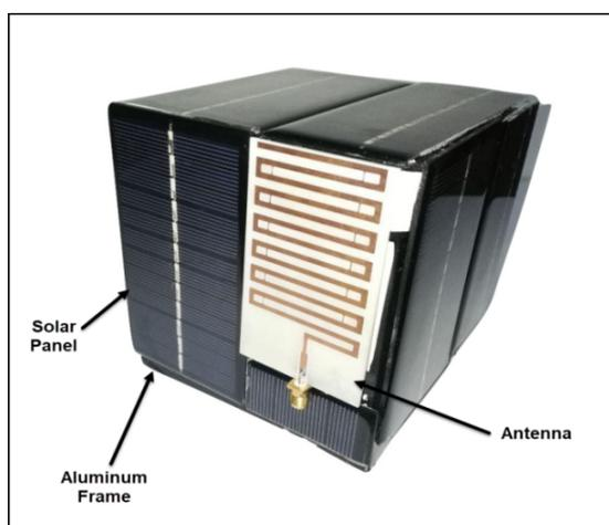
Figure 18: The fabricated antenna with 1U CubeSat.
