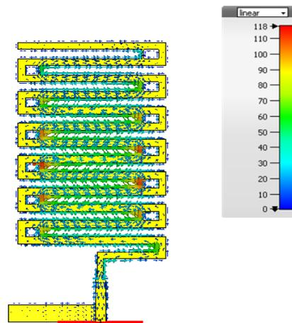
Figure 16: The surface current of the proposed antenna.
