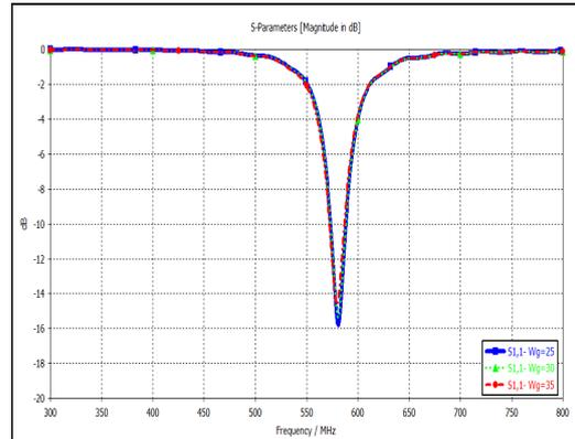
Figure 7: The effect of the ground plane width on the return loss.
