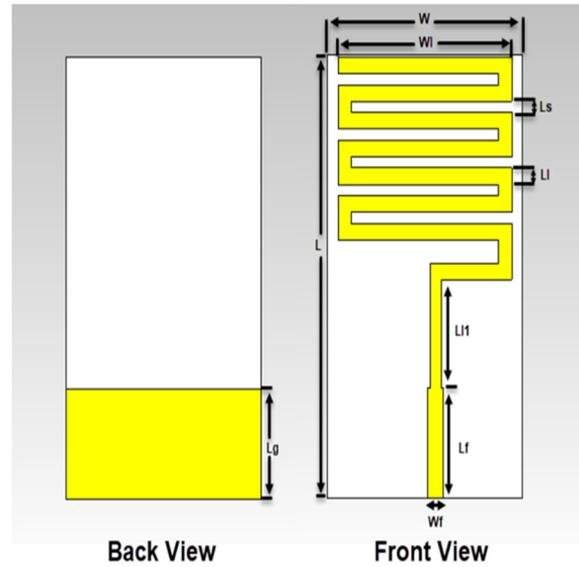
Figure 4: The primary design of meander line monopole antenna.
