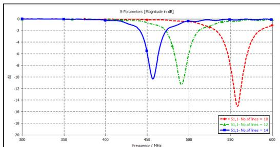
Figure 8: The effect of increasing the number of lines on the return loss.
