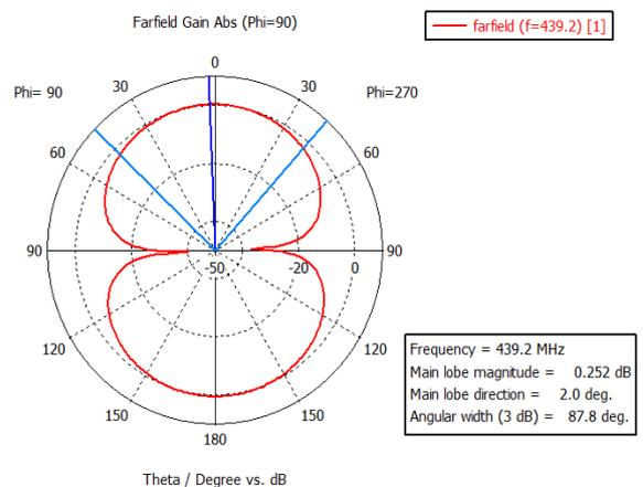
Figure 14: 2-D pattern of the far field directivity of the proposed antenna.
