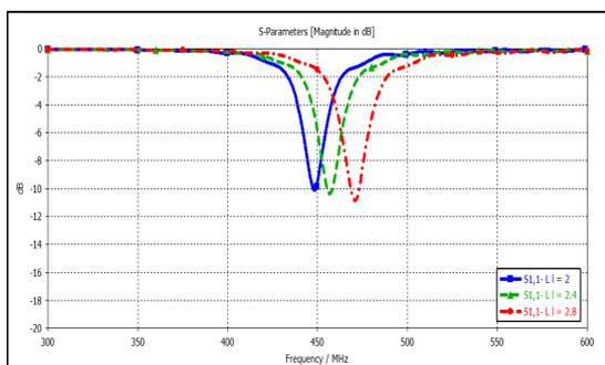
Figure 9: The effect of changing the line width on the return loss.
