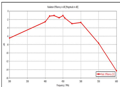
Figure 13: The radiation efficiency of the proposed antenna.
