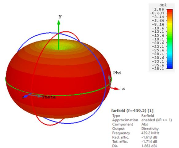
Figure 15: The 3-D pattern of the far field directivity for the proposed antenna.
