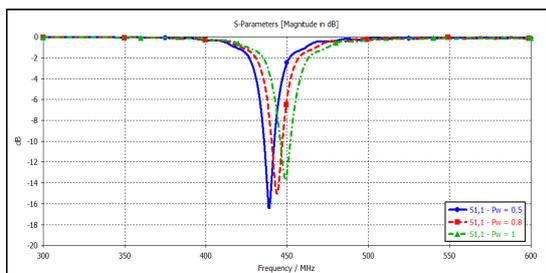
Figure 10: The effect of changing the thin pins width on the return loss.
