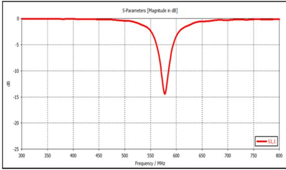
Figure 5: The return loss of the primary designed antenna.
