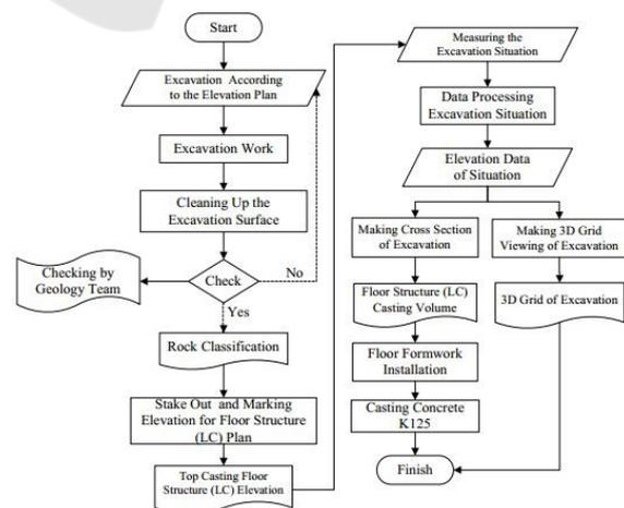
Figure 4: Work flow chart of floor.
