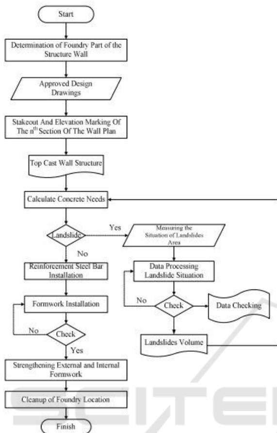
Figure 7: Structure work flow diagram.
