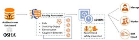
Figure 4: The 4D-BIM-based RTSP framework.
