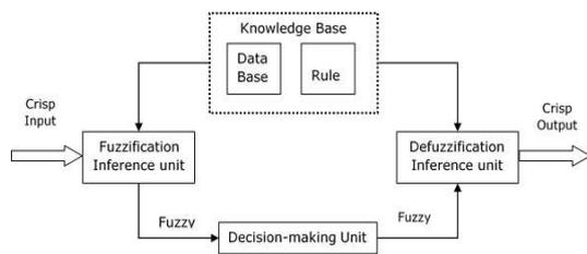
Figure 3: Block diagram of fuzzy interference system.
