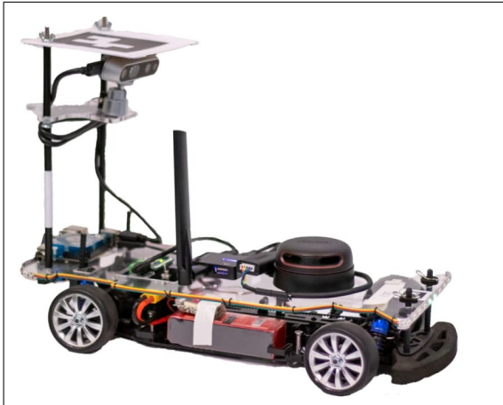
Figure 1: AutoMiny: a model car developed at Dahlem Center for Machine Learning and Robotics at Freie Universität Berlin.
