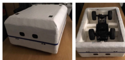
Figure 1: Scaled radio-controlled car with the casing inspired by the looks of a MiR100.
