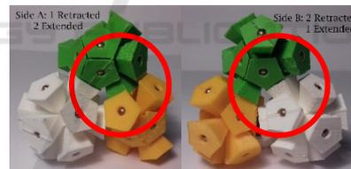
Figure 5: Craters - A crater formation of *2E1R Arms* is evident on Side A and a *R1E Arms*, crater is visible on Side B.
