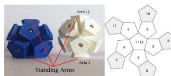
Figure 2: Root position – (a) root position with standing arms retracted & extended indicated by the red lines, (b) Facet / Arm allocation.
