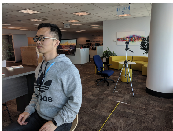
Figure 6: Quantifying air as a touch cue experimental setup. Observers sat in a chair at a measured distance from the haptic air device and estimated the time it took for them to start and stop feeling the air signal.
